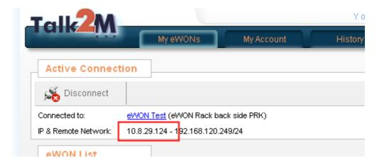
3. Open eBuddy and launch the "Upgrade firmware" wizard. Use the VPN IP address of the eWON.
