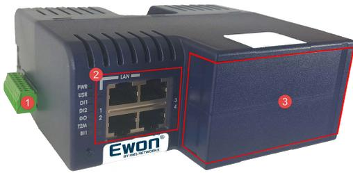
**Fig. 2 Modular Concept of the Flexy 205**
