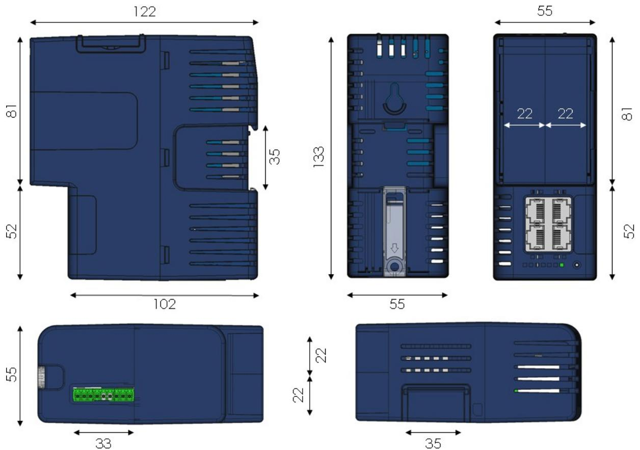
Figure 2. Mechanical Dimensions
