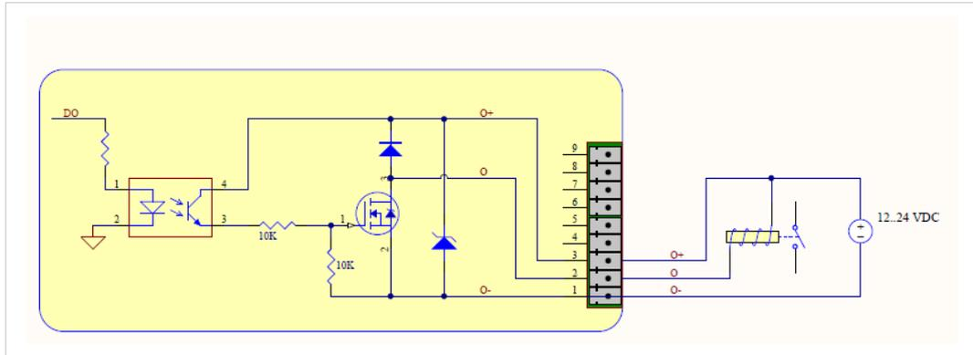
Fig. 14 External wiring for the Digital Output
