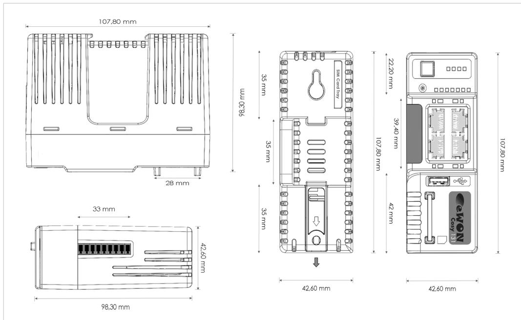
Fig. 5 Mechanical dimensions of the Ewon Cosy 131
