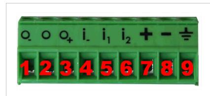
Fig. 12 Connector pinout
