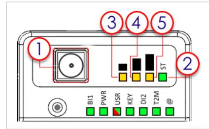
**Fig. 10** Status LEDs representation – Cellular model
