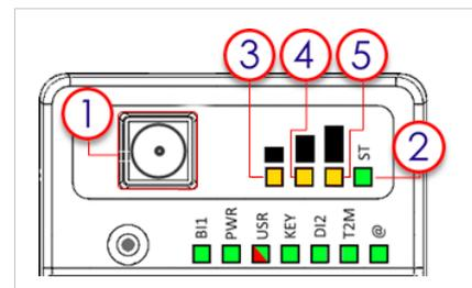
**Fig. 9** Status LEDs representation – Wi-Fi model
