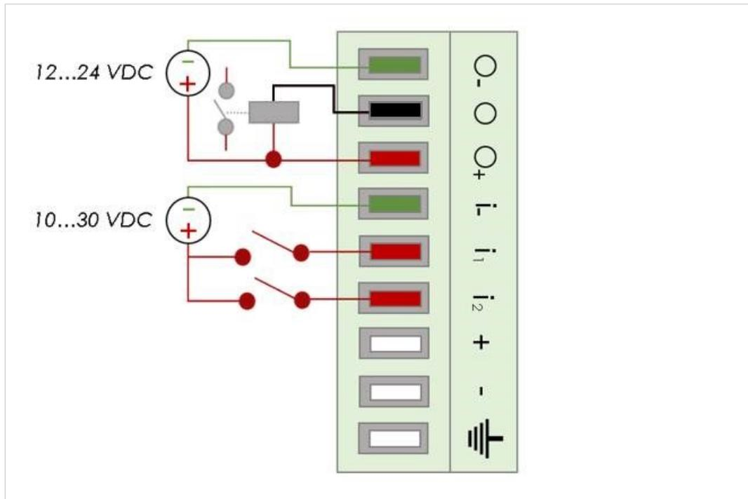
Fig. 13 Current scheme of the main connector
