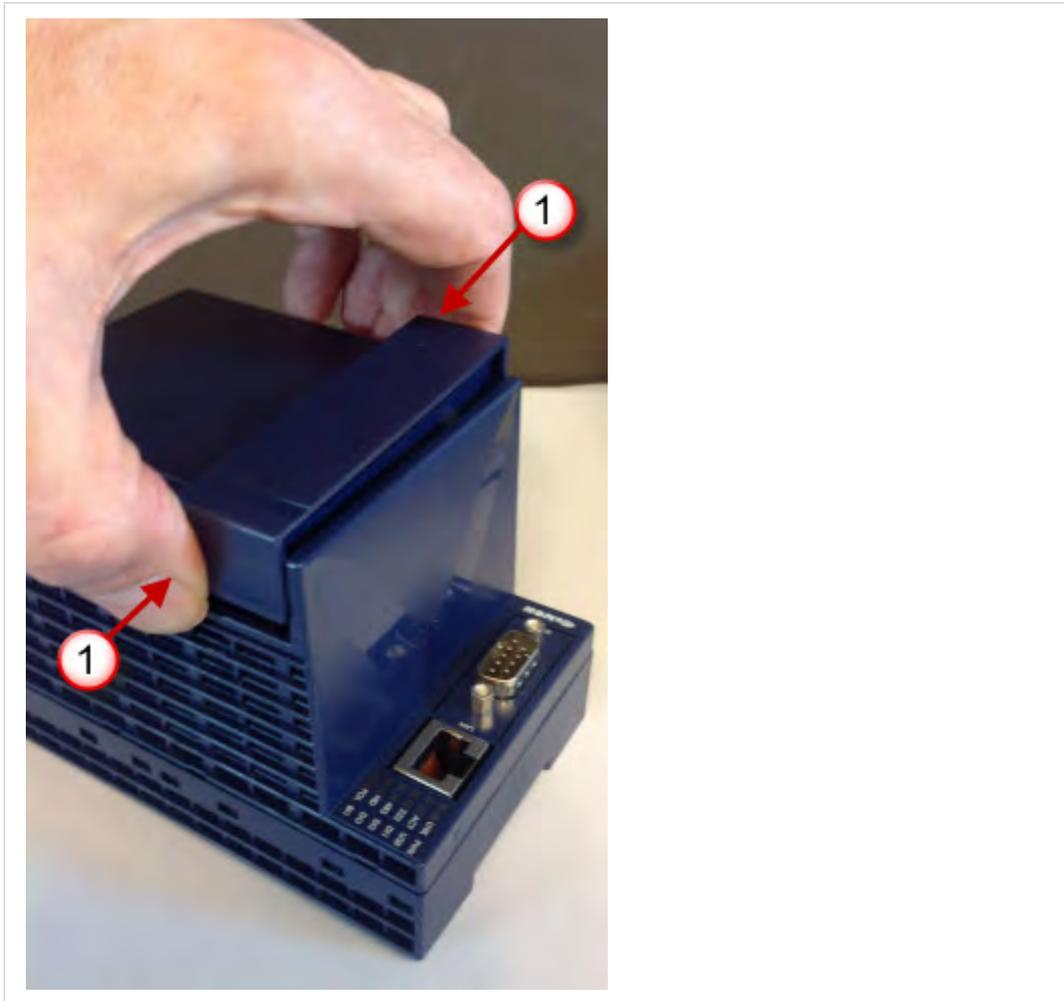
**Fig. 9 Remove the slot fillers**
