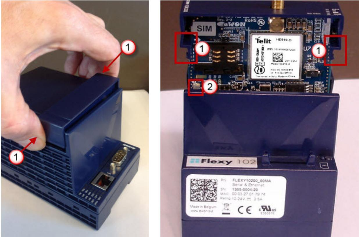
Figure 6. Remove the slot fillers
