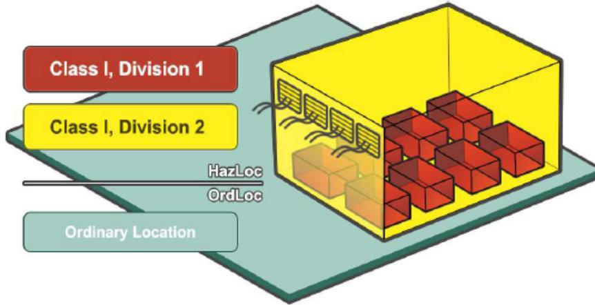
The standard FLA 3301 - 2 Serial Ports extension card, can only be placed and used in the green area: OrdLoc.
