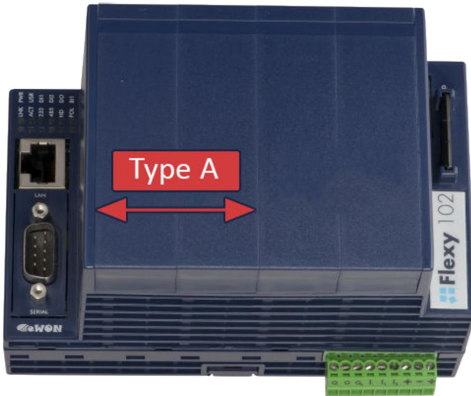
Figure 5. Position of the “A” Slots on a Flexy 10x & 20x.
