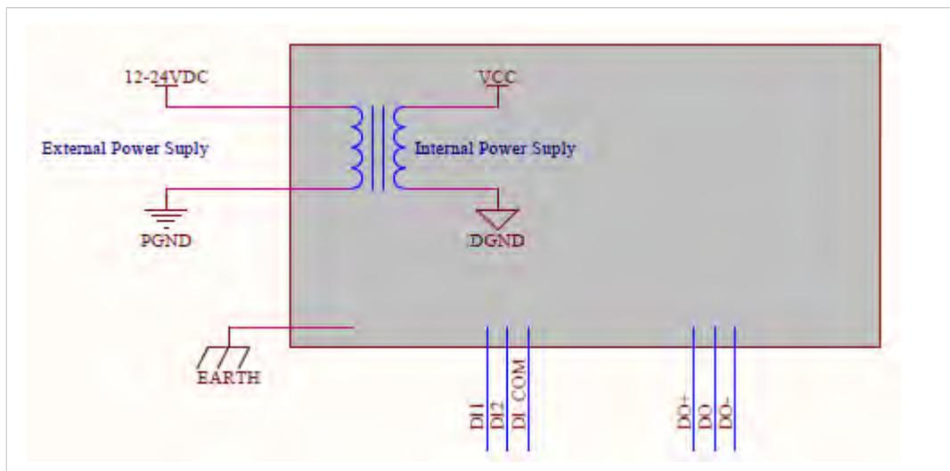
Fig. 22 Isolation Scheme for the Base Unit
