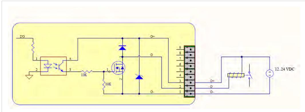
Fig. 21 External wiring for the Digital Output
