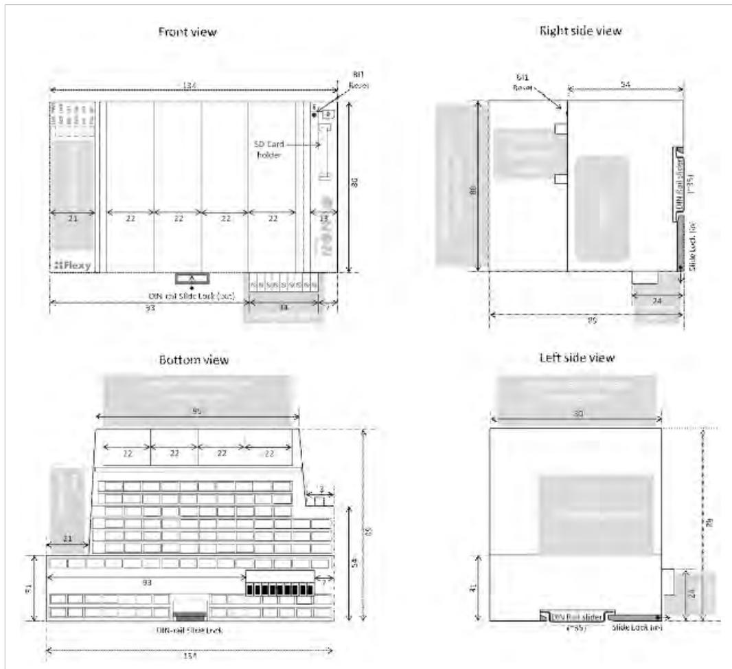
**Fig. 6 Mechanical Dimensions**
