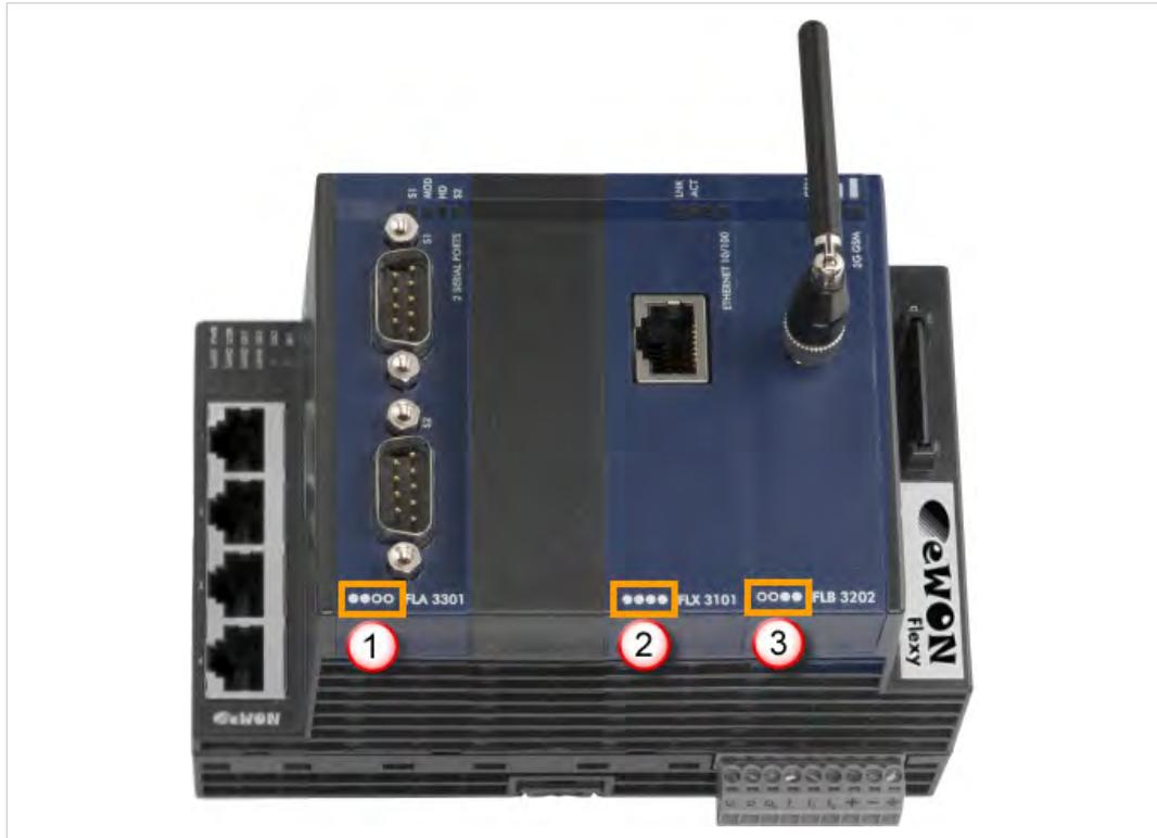
Fig. 16 Slot Compatibility Markings
