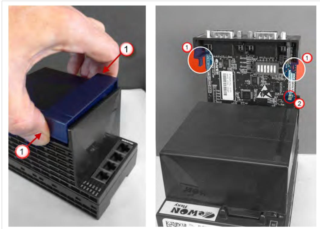
Fig. 17 Slot Removal
