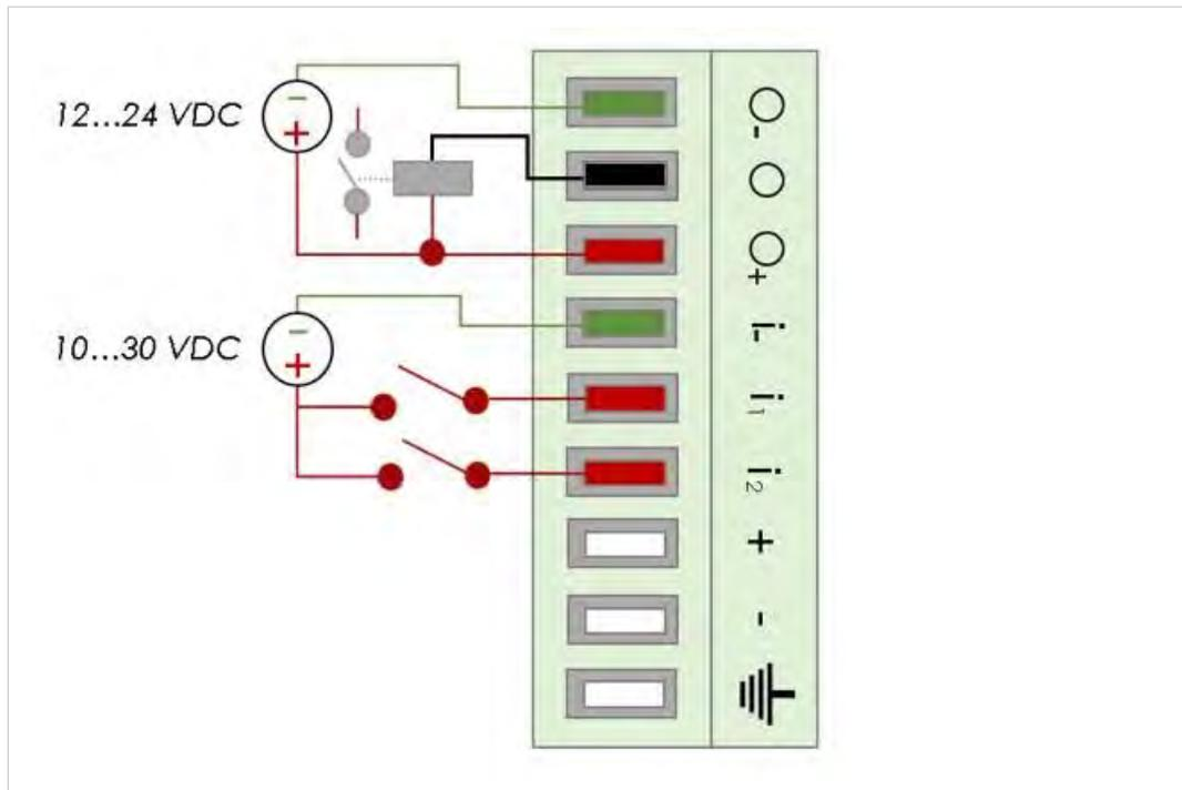
Fig. 20 Current scheme of the main connector
